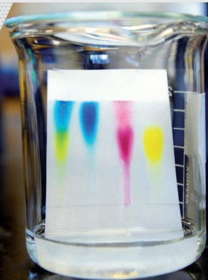
The separation is based on adsorption, partition, ion-exchange or on a combination of these mechanisms and is carried out by migration of solutes (**solutions of analytes**) in a solvent or a suitable mixture of solvents (**mobile phase or eluent**) through the thin-layer (**stationary phase**).
