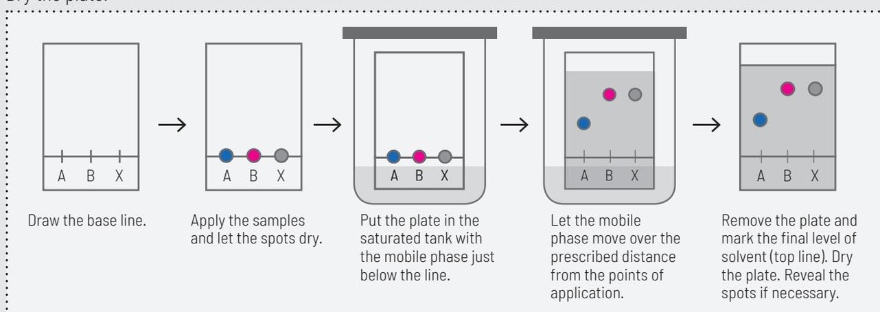
After the experiment, the spots are visualized. Often this can be done by simply projecting ultraviolet light onto the sheet; the sheets are treated with a phosphor, and dark spots appear on the sheet where compounds absorb the light that strikes a certain area. Specific reagents can also be used to visualize spots.
