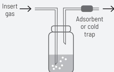
**Static head-space** injection systems include a thermostatically controlled sample heating chamber in which closed vials containing solid or liquid samples are placed for a fixed period of time to allow the volatile components of the sample to reach equilibrium between the non-gaseous phase and the vapor phase. After equilibrium has been established, a predetermined amount of the head-space of the vial is flushed into the gas chromatograph.
