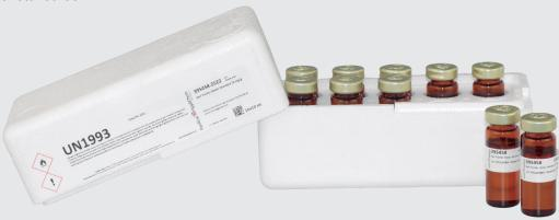
These standards are used to calculate the titer of AQUAMETRIC® Karl Fischer reagents for the volumetric titration and also to check the reliability of water determination using the coulometric method. AQUAMETRIC® Karl Fischer water standards are traceable to NIST SRMs and make the work of the laboratory staff much more reliable.
