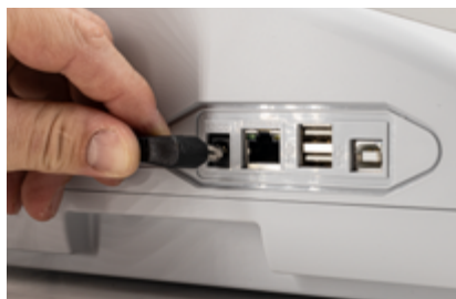
Fig. 2: Connecting the power supply
