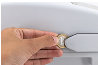
Fig. 1: Removing the interface cover
